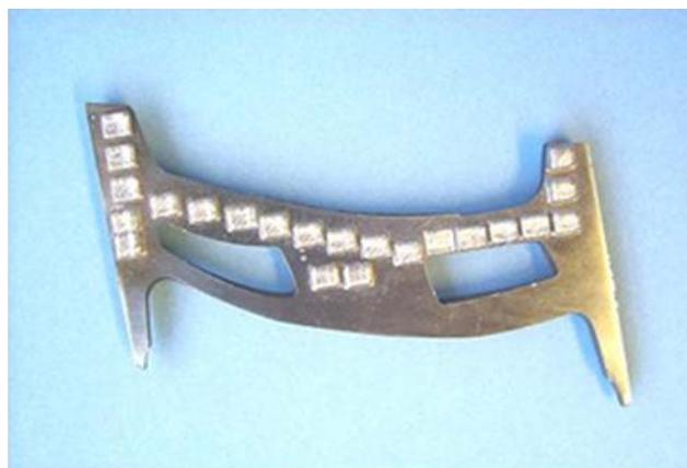
**Fig. 1** A GTD-111 test coupon showing the deposit areas
